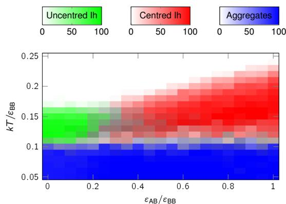
**Fig. 3** The yields of centred and uncentred icosahedra after  $10^6$  MC cycles as a function of  $\varepsilon_{AB}/\varepsilon_{BB}$  and temperature for a system of 120 B particles and 10 A particles at a density of B particles of  $0.15 \sigma_{BB}^{-3}$ , where  $\sigma_{pw} = 0.35$  and  $\sigma_{AA}/\sigma_{BB} = 0.95$ . Definitions of icosahedra and aggregates are the same as in Figure 2.
