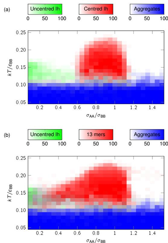
**Fig. 4** The percentage yields of (a) centred icosahedra and (b) 13-mers after  $10^6$  MC cycles as a function of  $\sigma_{AA}/\sigma_{BB}$  and temperature for a system of 120 B particles and 10 A particles at a density of B particles of  $0.15 \sigma_{BB}^{-3}$ , where  $\sigma_{pw} = 0.35$  and  $\varepsilon_{AB}/\varepsilon_{BB} = 1$ . The definitions of icosahedra and aggregates are the same as in Figure 2, and 13-mers are simply clusters with 13 particles.
